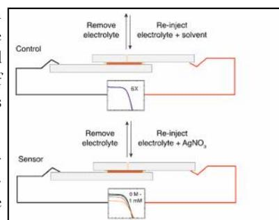
**Figure 2:** Schematic of the testing protocol for the control and sensor tests performed
