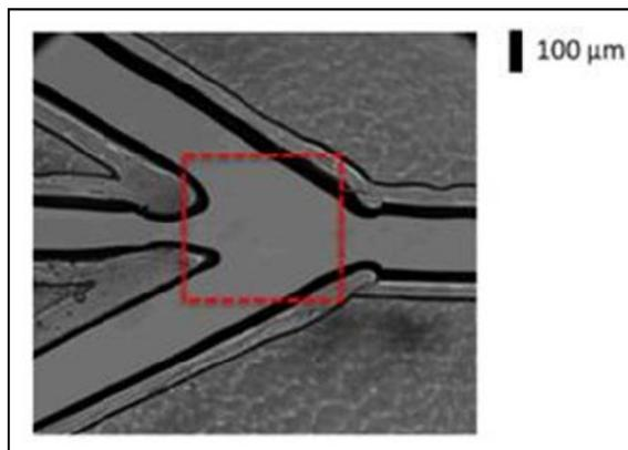
Microfluidic mixer utilizing mid-infrared hyperspectral imaging detection
