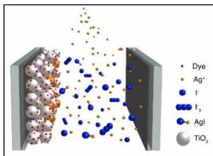
**Figure 1:** Schematic of a dye sensitized solar cell based silver ion sensor
